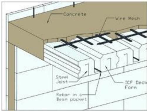
Cutaway view of an ICF floor on ICF walls.
