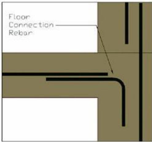
Section view of a removable forms floor on removable forms walls.
